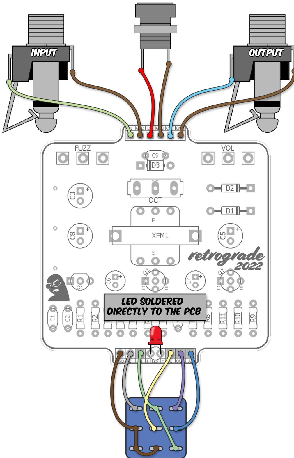
The In and J1 connections were accidentally transposed on the PCB so you will need to follow this diagram for proper bypass.
