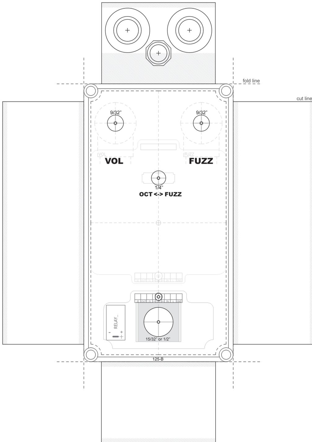
Use this template for “Softie3” relay bypass. Note the different bypass LED location. The drill location for the bypass switch is the same.
