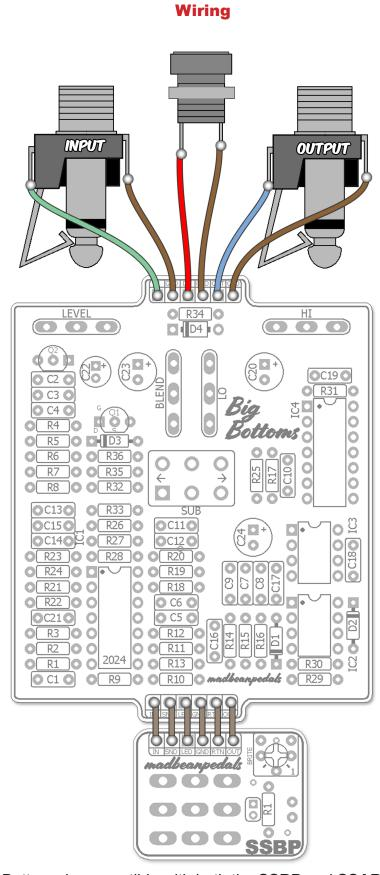
The BigBottoms is compatible with both the **SSBP** and **SSABP** bypass boards available at madbeanpedals. The wiring is the same for both.
