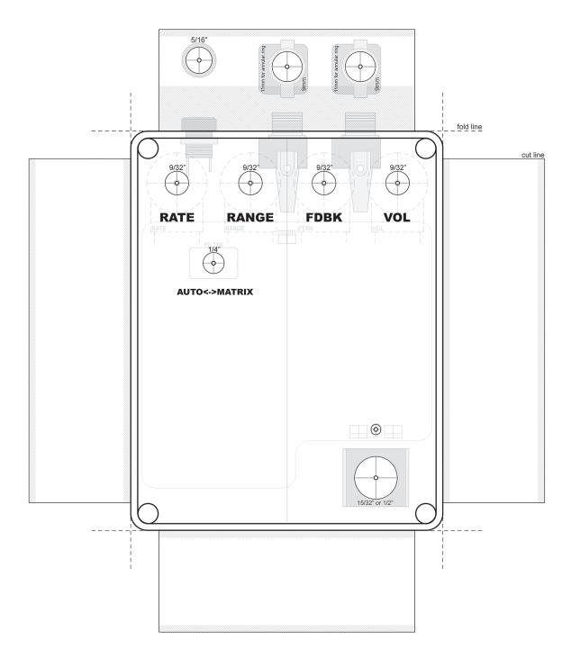
The I/O jacks are placed this way to keep them as far away from the LFO as possible (to avoid any noise or ticking).
