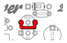
You only need to use the 78L15 regulator when using an MN3007 *and* 18v power supply. For all other permutations, omit the regulator and jumper the outer pads of the REG on the PCB as shown above.
