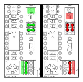
When using the MN3007, set the jumpers as shown in green. For the MN3207 or v3207, follow the jumpers in red. The jumpers determine which pins get power and ground and also what the Vgg voltage will be for the two different BBD technologies.
