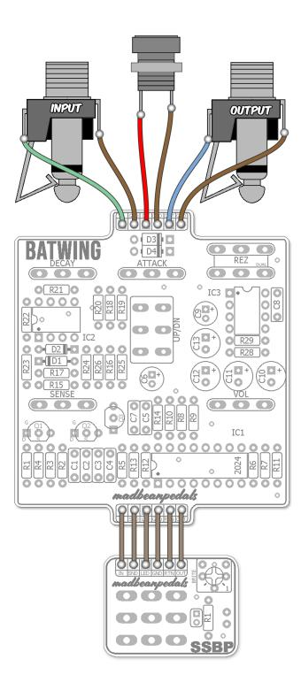
The Batwing24 is compatible with both the **SSBP** and **SSABP** bypass boards available at madbeanpedals. The wiring is the same for both.
