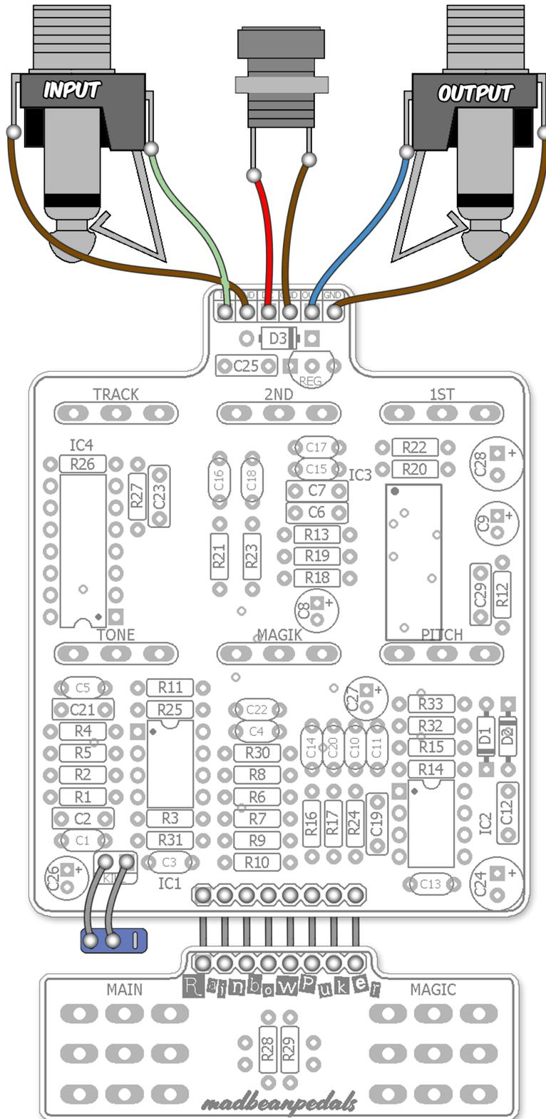
An 8-pin, 1" ribbon cable is recommended for soldering the connections between the two PCBs.
