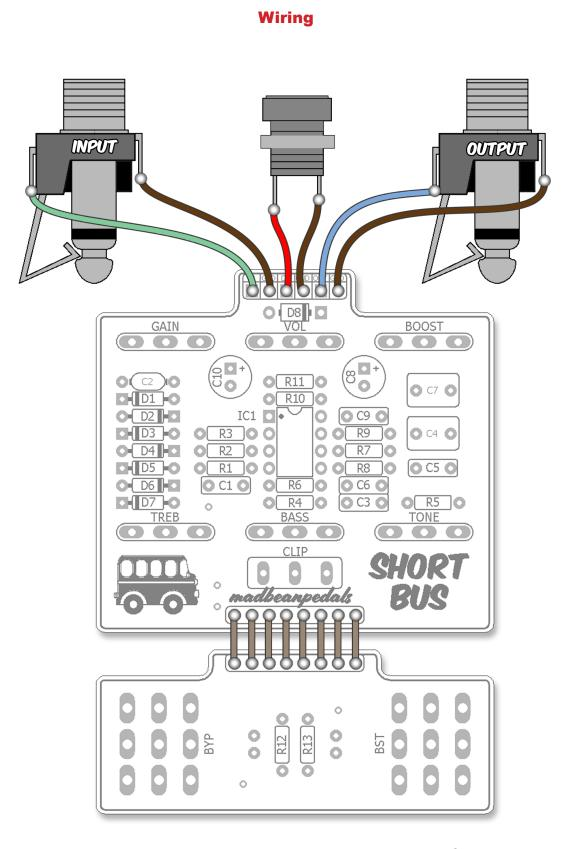
The 3PDT and LEDs are soldered directly to the bottom of the daughter board.
