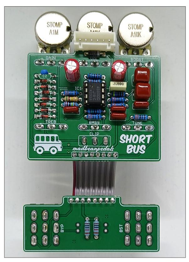
At the time of this build, I had no PCB mounted 500kA pots. So I used a 1MA pot and put a 1M resistor in parallel with it.
