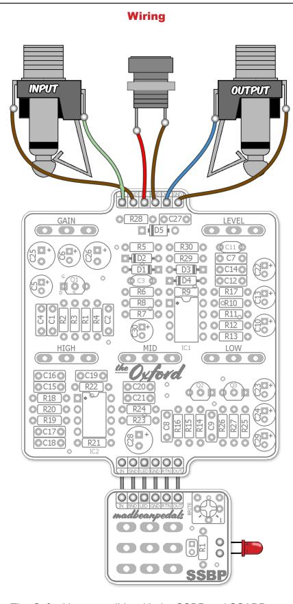
The Oxford is compatible with the SSBP and SSABP bypass boards offered at madbeanpedals. Both use the same wiring.
