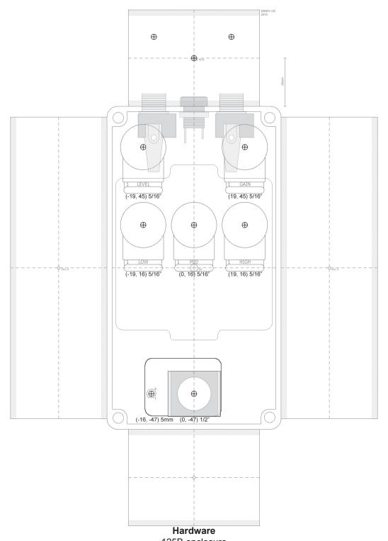
125B enclosure Lumberg 1/4" Compact mono jacks Slim 2.1mm DC jack Standard 3PDT footswitch
