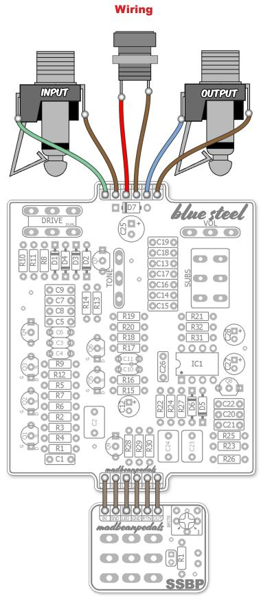
The BlueSteel24 is compatible with both the **SSBP** and **SSABP** bypass boards available at madbeanpedals. The wiring is the same for both.
