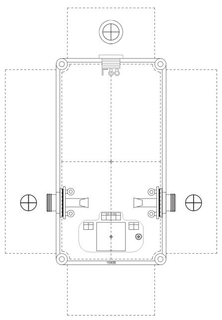
This template shows a typical layout for a 1590B using the 3PDT-03.
