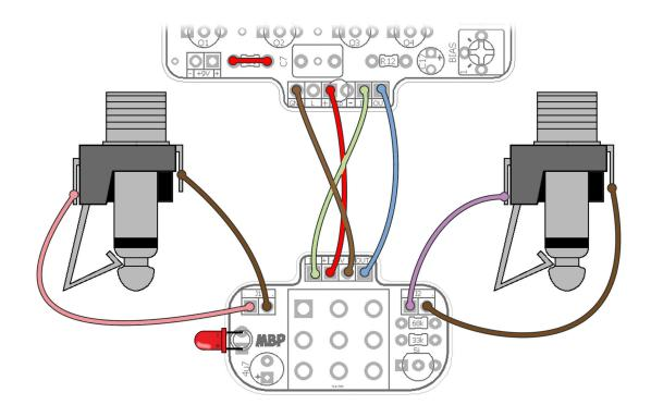
This diagram shows a typical madbeanpedals project and one way the 3PDT-03 board could be wired. Since almost all mbp projects include a bypass LED on it, we need to..err, bypass that!
