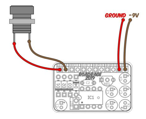
For -9v operation only you can omit D3, D4, C3, C4, C7 and the regulator. Here the red wire is ground and the brown wire is -9v.
