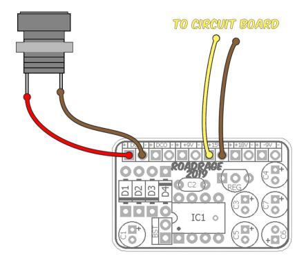
For +15v (regulated) or +18v (unregulated) omit C5 and C6. You can put a jumper between the + and - pads of C6 to ground pin5 of the charge pump. This is not required, but it is good practice when you are not using the inverter pin.
