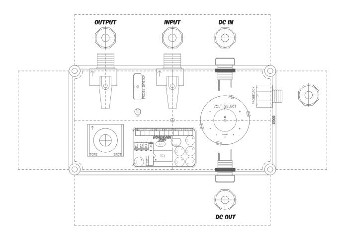
One point of caution: with the -9v option on the rotary switch it's possible to be careless and send -9v to a +9v build or circuit on your breadboard. If you want extra insurance, wire the -9v output to another DC jack and just plug that in when you need it.
