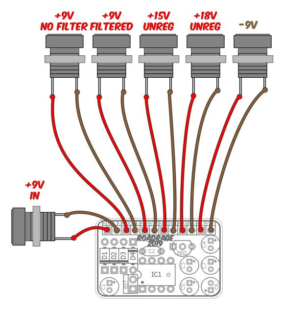
Another use for the RoadRage is as a power supply for breadboarding. This gives you the additional option of +9v unfiltered or +9v filtered (IOW, with power decoupling). There are some cases where one is better than the other.
