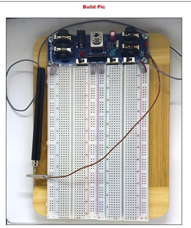
I used a cheap cutting board from Amazon to mount everything. For the PCB, I used #4 sheet metal screws to secure it to the cutting board. I also used stick-on rubber feet in the corners on the bottom.
