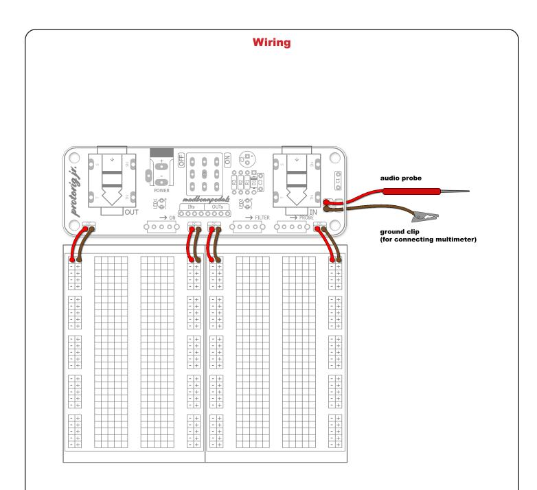
Note the "+" and "-" orientation of the breadboards.
