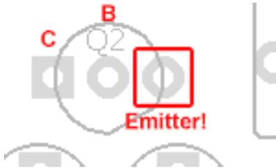
The 2n3565 has a flattened end on the mushroom style casing. The flattened part indicates the emitter. Be sure to put the transistor in the right way!
