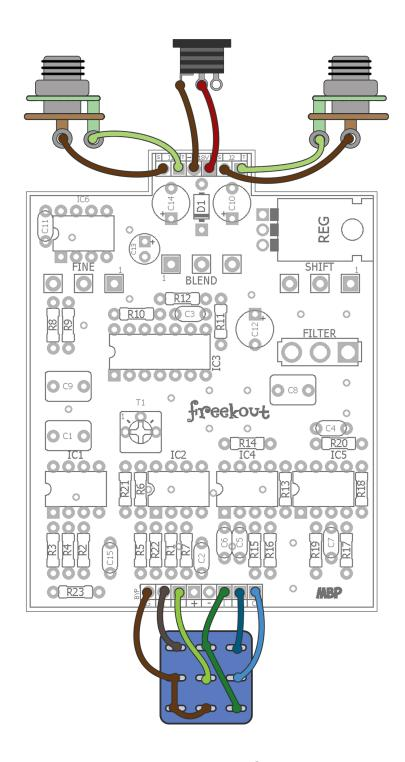
The indicator LED can be mounted directly to the PCB (+ and – pads on the bottom row).
