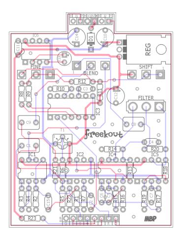
This project requires an 18v 100mA (or more) center tip negative power supply. I recommend the Dunlop 18v wall-wart.
