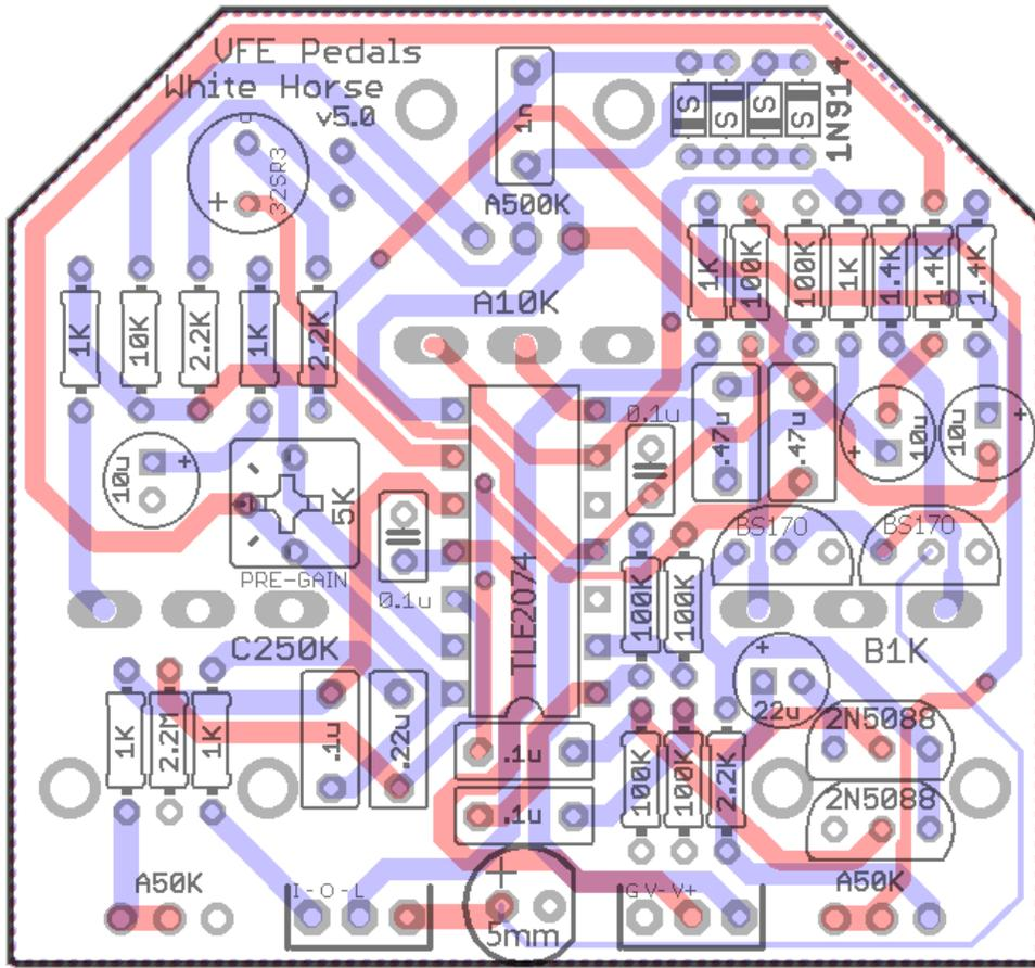
*This image shows ver.5 instead of ver. 4.2 (the one I have). There are two differences: the three 10uF BiPolar caps are show as electrolytic instead of film caps and the two BS170 transistors used for clipping were changed to four 1n914. If you want to use the clipping from ver.5 in your build, see the last page of this document.*
