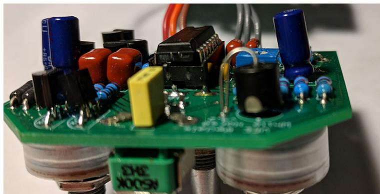
Install the NSL-32SR3 optocoupler as shown here. The dot indicates the cathode of the internal LED. The lead spacing is a little small so you will have to bend the pins inward slightly (you can just make that out in the pic at the top of this page). I do not recommend trying to roll your own optocoupler. Stick with the NSL.
