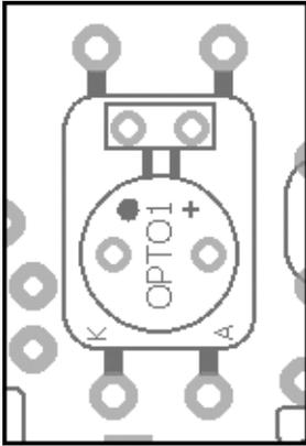
Opto1 has solder pads for both the VTL5C9 and NSL32. I recommend using the 5C9. It is a more expensive parts, however, having tested both devices in this build the 5C9 does a better job of pulling out finer detail in some of the more esoteric waveforms in Bank2. If you cannot get the VTL5C9, use the **R3** version of the NSL32.
