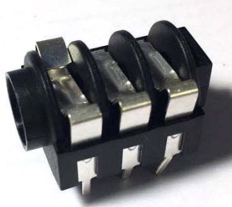
A "sleeve make" jack – the sleeve contacts the switched pin to make the DC Ground connection.
