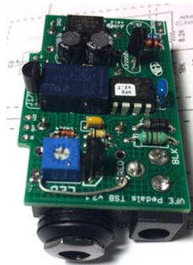
Here the sleeve and switched pin are shorted together with a buss wire for DC ground.
