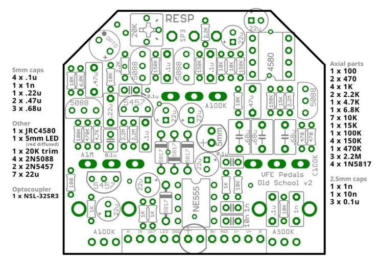
Note: Use the values listed on the image above – not the values indicated on the silk-screen of the PCB. Some values changed over time in the VFE product cycles.
