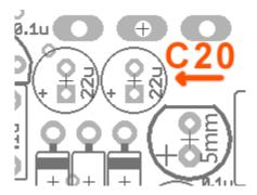
The NE555 is used as a charge pump to create around 22v as the supply on the audio path. A 35v rated 22uF for C20 would be ideal, but if you only have 25v rated caps stick with that. Space is pretty tight in that area.
